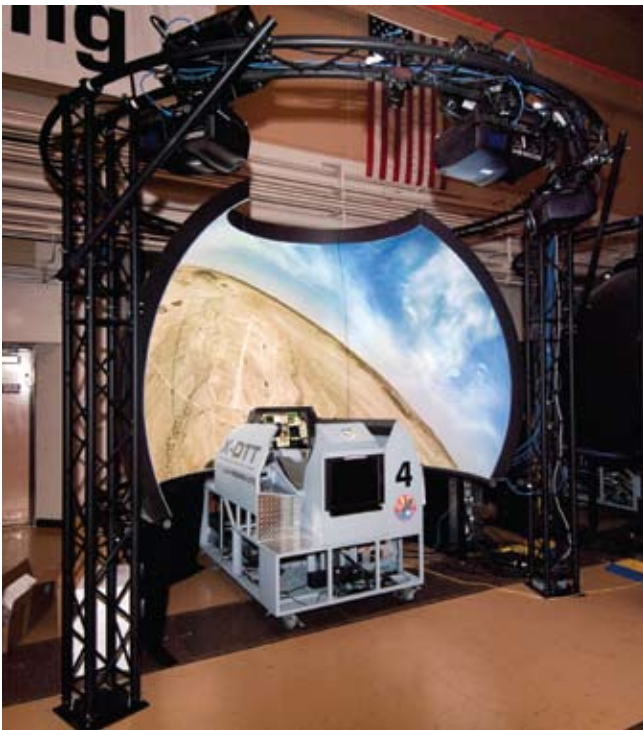
One of the F-16 X-DTT simulators at AFRL using MetaVR multi-channel visual systems. (Note that the seams that appear in this test installation of the dome will be eliminated in the final installation.) Image courtesy of Air Force Research Lab (AFRL).
