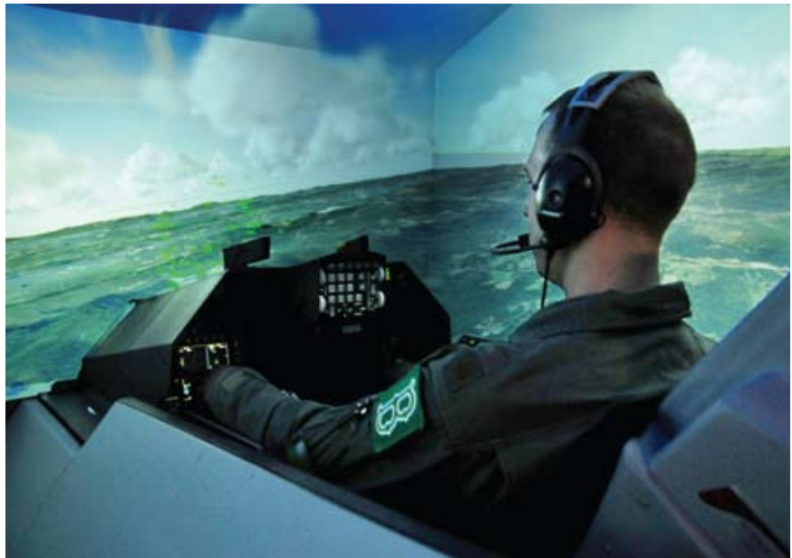
One of the 4 cockpit simulators at the new F-16 Mission Training Center, located at the VT ANG base, Burlington, VT. The multi-channel synchronized view, driven by VRSG, is rendering the VT virtual terrain built by MetaVR. Photo courtesy of SSgt. Dan DiPietro, 158 FW, Vermont Air National Guard.
