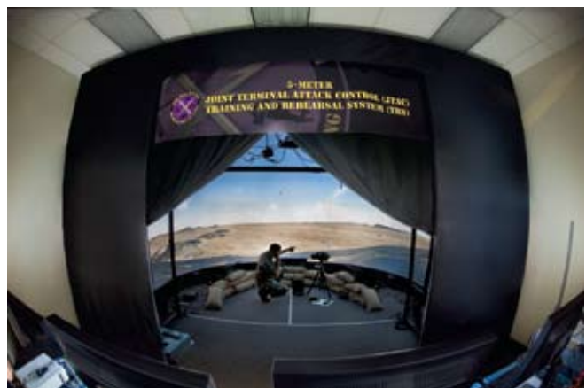
The deployable JTAC Virtual Trainer Dome using MetaVR VRSG software. Image courtesy of AFRL, Mesa, AZ.
