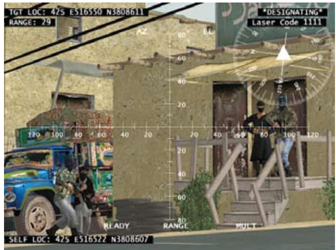
VRSG real-time screen capture of a scene on MetaVR's virtual Afghanistan, which the operator on the left sees when looking through the simulated laser designator with embedded 3D graphics hardware. With information such as the laser code, the target location, and the compass rose, this view is the same view as seen in the FPS desktop-based JTAC simulator. The desktop and dome simulators produce the same designator view.
