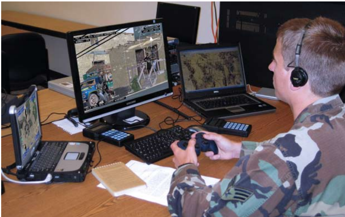
A JTAC trainee at the Air National Guard Simulation Lab running MetaVR VRSG and Afghanistan database (on the middle computer). On the left is a ROVER IV, and on the right is FalconView map of the same area. On the desk are ASTI VOIP handheld terminals that simulate radios.
