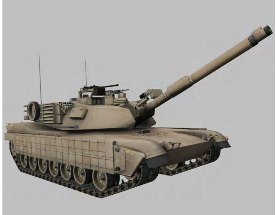
MetaVR's M1A2 TUSK model, which is comprised of 12,505 polygons and 16 photo-specific textures (112 MB of textures). The images on the left show a photograph of the turret area of the actual vehicle (topmost), with textured and wireframe views of the same area on the model.
