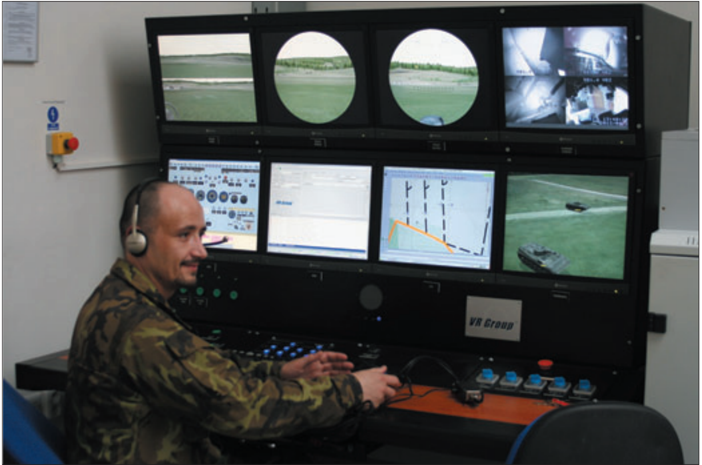
A Czech Army instructor demonstrates the instructor operating station for the BMP 2 simulators.
