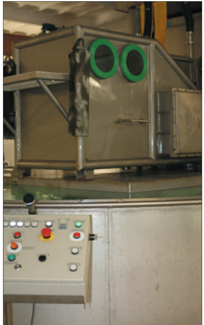
The underwater emergency evacuation trainer showing the vehicle cab and the operator's position. The major safety feature is the ability of the instructor to rapidly raise the cab in the event of a problem.
