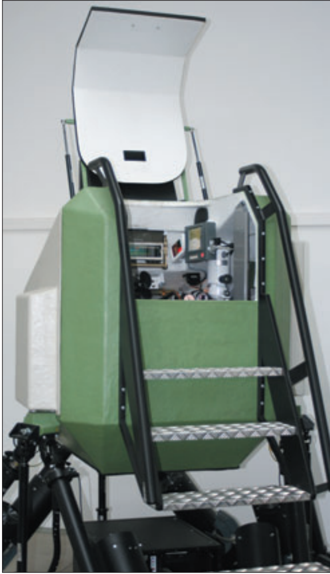
The driver's compartment of the Saab Czech Pandur AIFV simulator. Such devices are referred to as Type One simulators.
