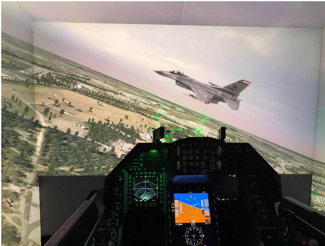
Image: F-16 cockpit view of VRSG showing geospecific 3D terrain of Kelly Field, Lackland Air Force Base, built by MetaVR for the ANG. (Credit: US Air Force.)
