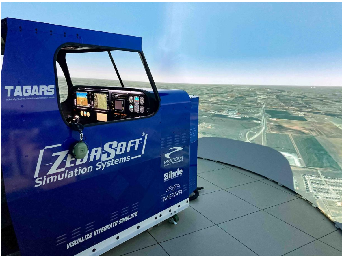
Image: VRSG provides the simulator’s out-the-window view over MetaVR’s round-earth geospecific 3D terrain of CONUS (Image courtesy of ZedaSoft).
